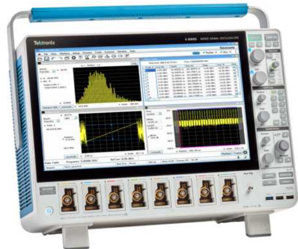
MSO68B showing SignalVu-PC pulse analysis running on the instrument
