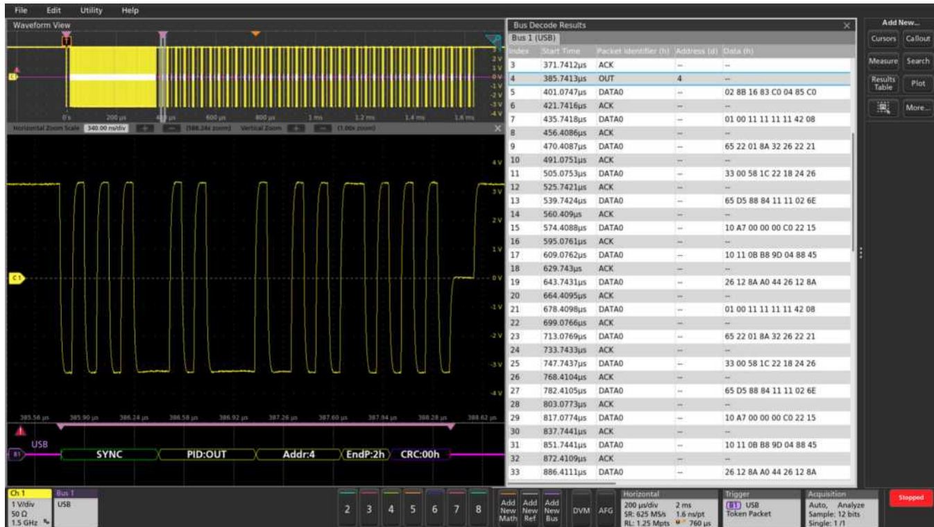
Triggering on a USB full-speed serial bus. A bus waveform provides time-correlated decoded packet content including Start, Sync, PID, Address, End Point, CRC, Data values, and Stop, while the bus decode table presents all packet content from the entire acquisition.
