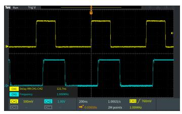
Measurements are transparent so waveforms are not obscured.
